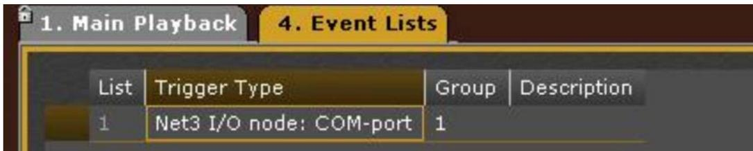
Once a Net 3 I/O Node:COM-port is inserted you are now able to open the event list by pressing [MODIFY] on the selected list #.
